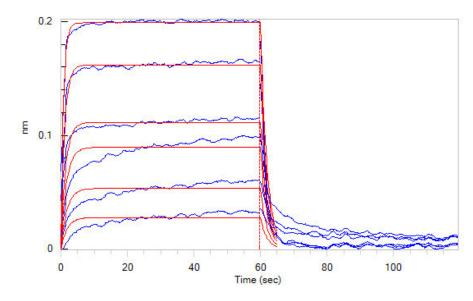
Loaded Mouse PD-L1, Fc Tag (Cat. No. PD1-M5251) on Protein A Biosensor, can bind Mouse PD-1 Protein, His Tag (Cat. No. PD1-M52H3) with an affinity constant of 2.5  $\mu$ M as determined in BLI assay (ForteBio Octet Red96e) (Routinely tested).
