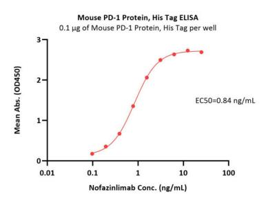
Immobilized Mouse PD-1 Protein, His Tag (Cat. No. PD1-M52H3) at 1  $\mu$ g/mL (100  $\mu$ L/well) can bind Nofazinlimab with a linear range of 0.1-2 ng/mL (QC tested).
